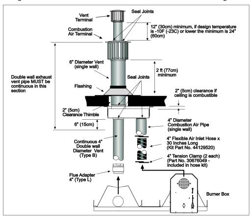
The figure below shows the connection details for vertical concentric vent through roof with STRAIGHT TUBES.
