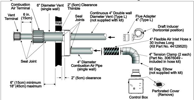
Below are typical arrangements for routing the concentric vent to the SIDE WALL.
